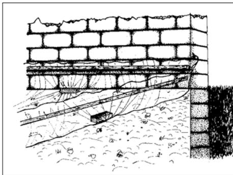
Figure 7 Crawl space air-vapor barrier
