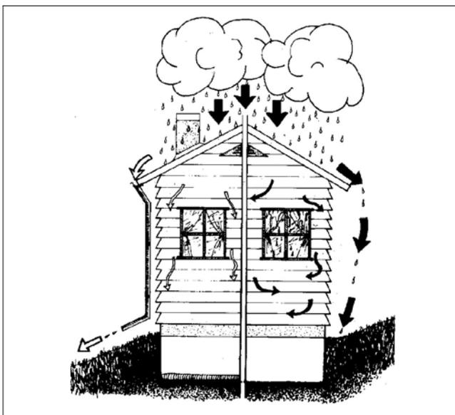
Figure 8 Gutters, a slope away from the house and drainage tile in the foundation keep the left side of the house dry. No gutters, a slope toward the house, and no drainage tile expose the right side to moisture damage.
