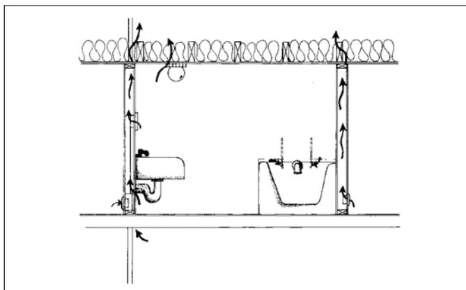
Figure 2 Attic bypasses for the bathroom
