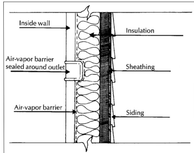
Figure 4 Air-vapor barrier placement
