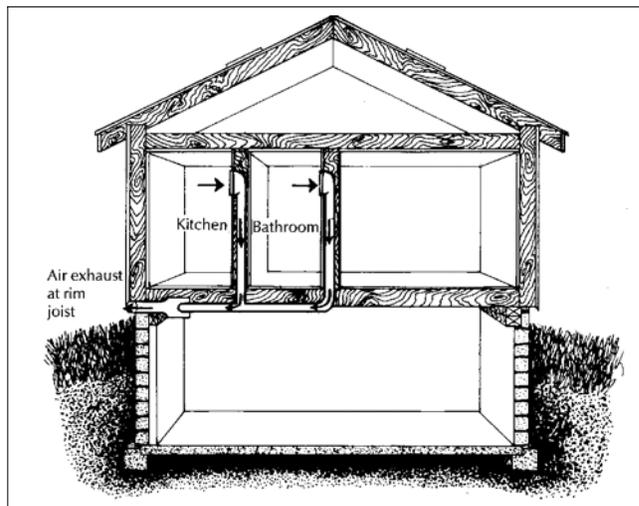
Figure 5 Mechanical ventilation
