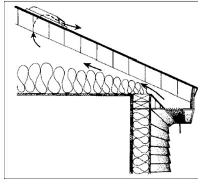
Figure 6 Mechanical ventilation
