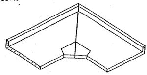
Notch and fit Diagonal Front With No Sink Diagonal face cabinet length must be less than 20" Front rolls come attached
