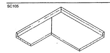
Different depth tri cove tops mitered together where 1 or both tops have a screwed on backsplash All are specials miters
