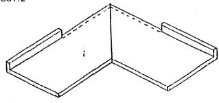
Notch and Fill-In Backsplash is removed, and top is filled in flat to Nose cap required when end of backsplash is exposed
