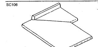
Tri Cove top mitered to island top 90, 22 1/2, or 45 degree, std. Miter any other degree is a special miter Nose cap required on end of backsplash
