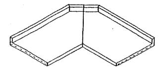
Diagonal Comer Wall Diagonal rolled splash is SCREWED on
