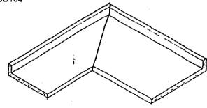
Different depth tri cove tops mitered together 90, 22 1/2, or 45 degree, std. miter
