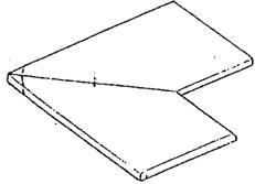
Equal depth island tops mitered together 90, 221/2, or 45 degree, std. miter Any other degree is a special miter
