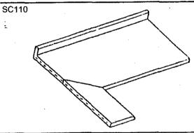
Tri cove top mitered to single roll top 90, 22 1/2, or 45 degrees, std. Miter Any other degree is a special miter
