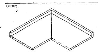
Equal depth tri cove tops mitered together 90, 22 1/2, or 45 degrees, std. miter Any other degree is a special miter
