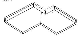
Chimney Notch Available with or without: L shaped square edge splash L shaped rolled splash (attached)
