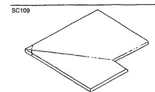
Different depth island top mitered together All are special miters Eased outside comer is recommended
