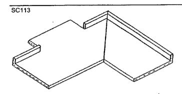
Notch and SCREWED on Backsplash -- Island Top is notched out and rolled backsplash is SCREWED on
